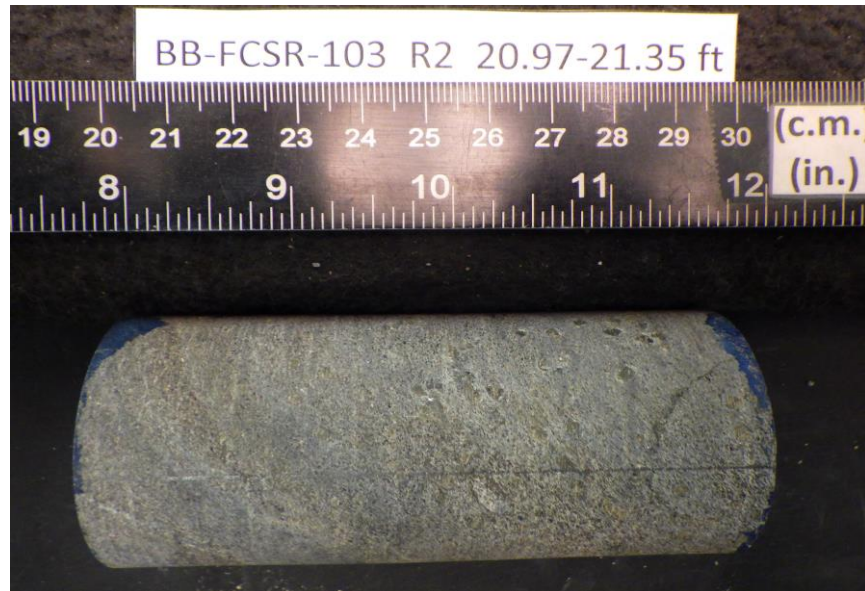
After cutting and grinding
